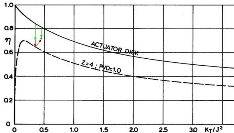
*Propeller efficiency in relation to efficiency of an actuator disc (illustration only)*
