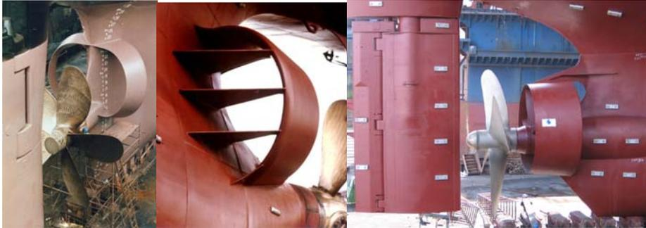
The above indicates that the working mechanisms of pre-ducts are complex and depend strongly on their design and mounting position. As a wake concentrator, pre-nozzles require a high wake to be effective, and thus these devices are found on high block vessels.
