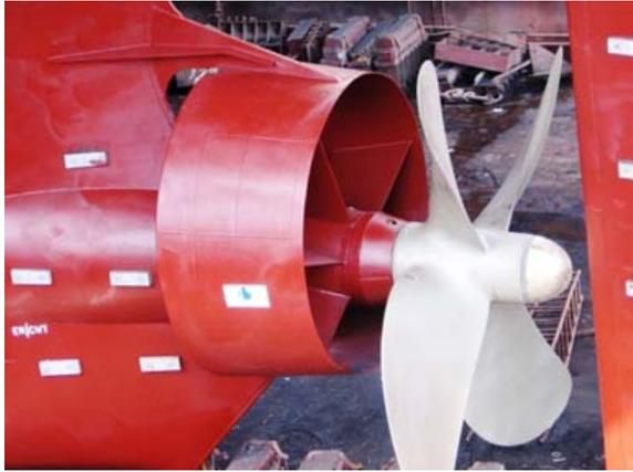
**Figure 1.** First installed full scale Mewis Duct<sup>®</sup>, STAR ISTIND, 45,000 tdw MPC, September 2009
