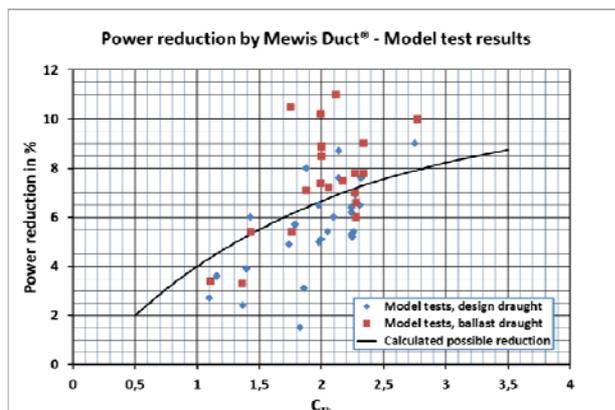
**Figure 2.** Power reduction by Mewis Duct<sup>®</sup>, model test results, average measured power reduction: 6.4 %
